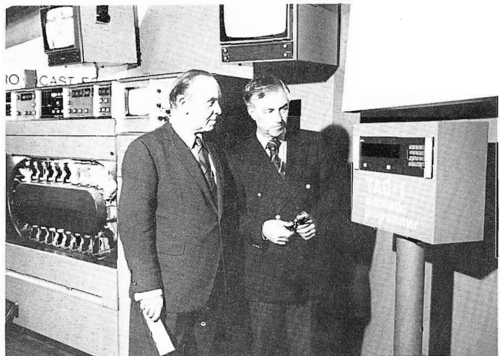
As many as 80 program segments can be sequenced automatically with the new TAC-1 Automatic Programmer. Sources can be tape, film or slide.
