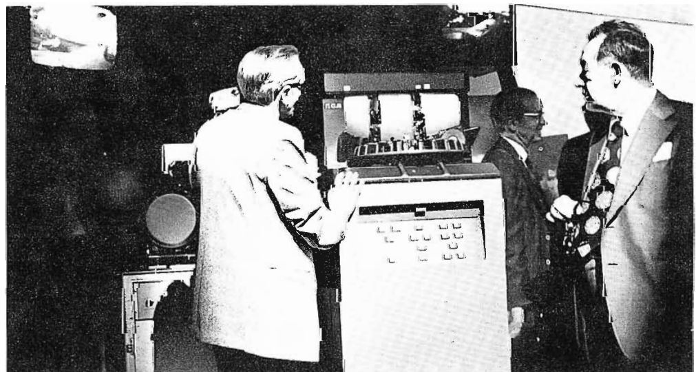
A major attraction at the show, the TCP-1624 can handle up to 24 film cartridges on a carousel tray. This unique system can broadcast a single spot or a sequence of spots in any combination, from 10 seconds to two minutes.
