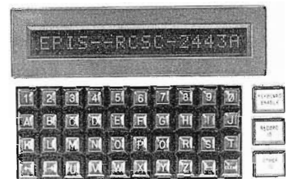
EPIS (Electronic Program Identification System) is an optional TCR-100 feature which displays an alpha-numeric identification of cued and on-air cartridges.
