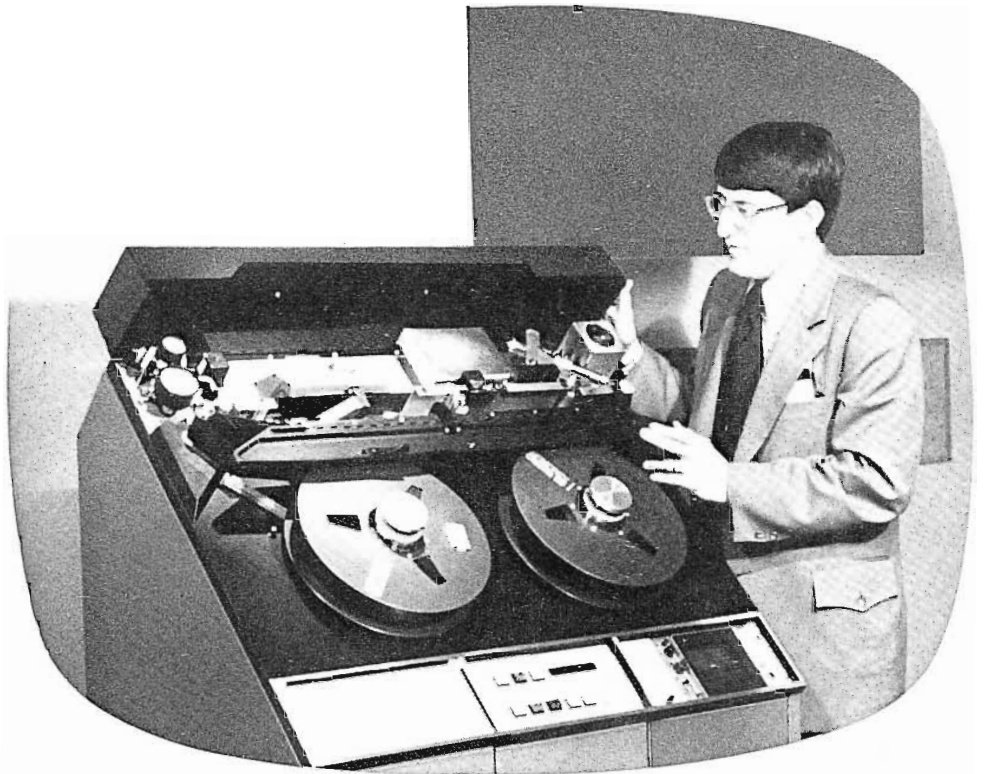
Introduced at NAB was the New Technology TR-600, a fresh departure among quad tape recorders. Smaller, lighter, and easier to operate, it includes numerous built-in features and operator aids such as drop-on loading.
