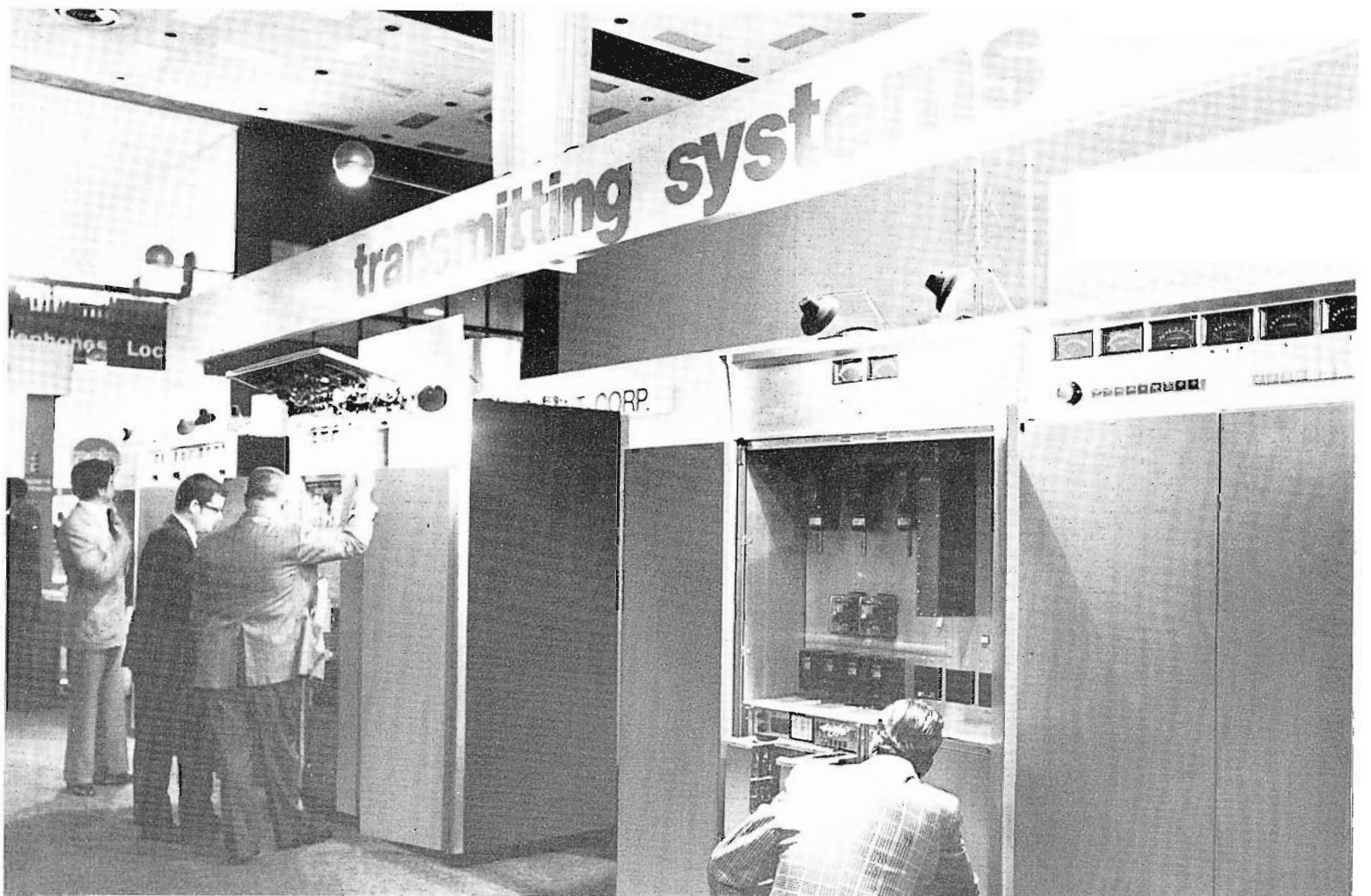
Three in a row. The TV Transmitter line-up at NAB included the TT-25FL lowband, the TT-25FH highband VHF systems, and the TTU-30C UHF which is solid state up to the final stage.
