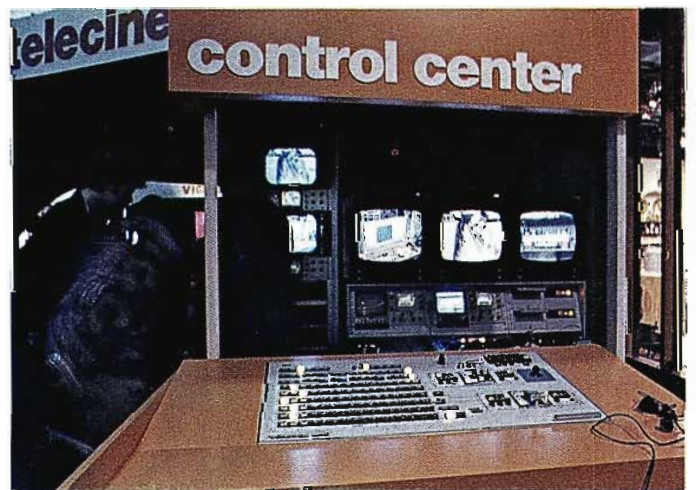
Along with the usual monitor displays, the Camera Control center demonstrated the compatibility and virtual interchangeability of Camera Control Units for the TK-45A and TKP-45 Cameras.
